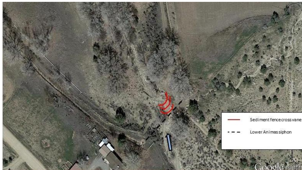
Figure 24. Lower Animas Siphon Erosion Control Conceptual Plan at Rabbit Arroyo
